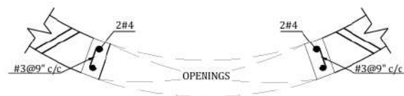
S-03 REINF. DETAIL FOR OPENINGS SCALE: 1/2"=1'-0"
